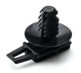
Connector Clip with Round Fir Tree, 0.7 - 4.0 mm Panel Thick., 6.0 - 6.7 mm Hole Dia, PA66HIRHS, Black, 5000/box
