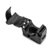
Bolt Mount Ratchet Clamp for Low Torque, 0.76 - 1.42" Bundle, 0.41" Hole, PA66HIRHSUV, BK, 25/bag
